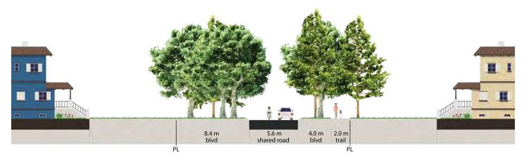
Figure 6.4: Lochside Drive with future separated pedestrian pathway
